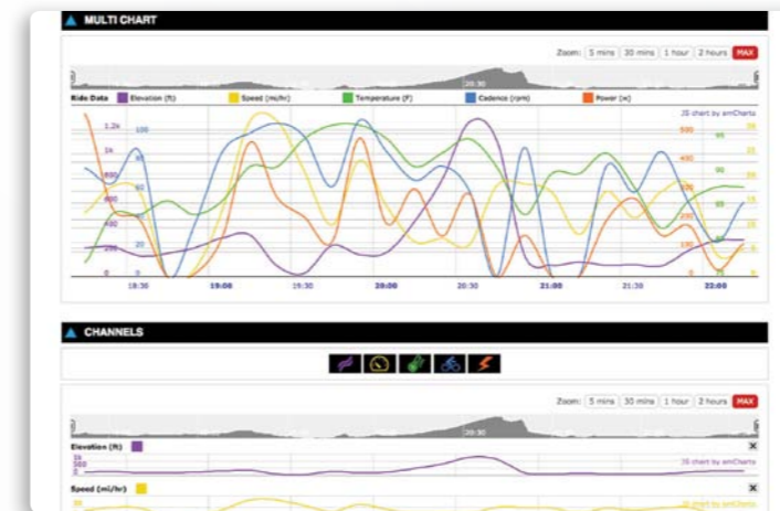
Detailed ride data can be viewed in the website's graphs. Each channel of data can be turned on or off, and information can be analyzed up to the second with the graph's high-zoom capabilities.
